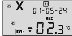
1 hour later the low alarm temperature duration triggers an alarm. The bell (Alarm) symbol is seen, buzzer triggers (audible).
